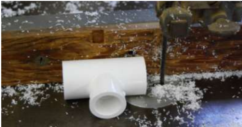
Cutting the tees on a bandsaw with a fence
